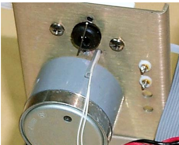
Figure 31 EN-SCI Model Z with OIF411 Temperature Sensor Assembled
