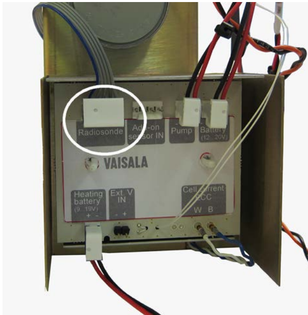
Figure 38 Connecting Radiosonde Cable
